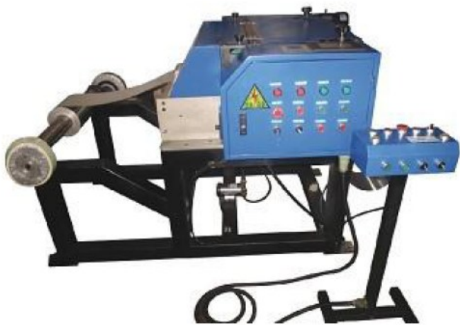
The Feeding Machine With Lubricated Oil System
